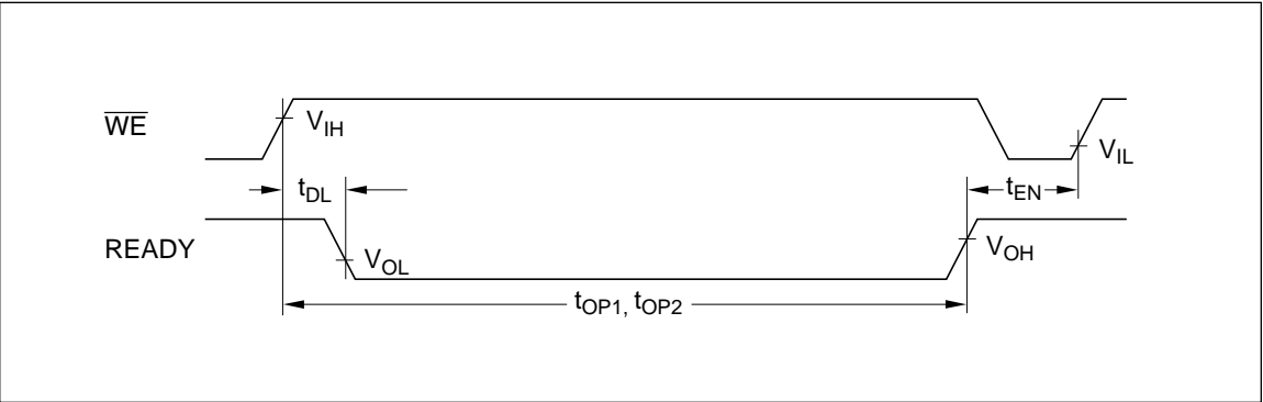
Figure 29 \overline{READY} Timing (When the \overline{READY} Output Is Always Available)
