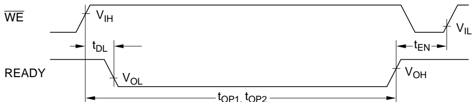
Figure 29 READY Timing (When the READY Output Is Always Available)
